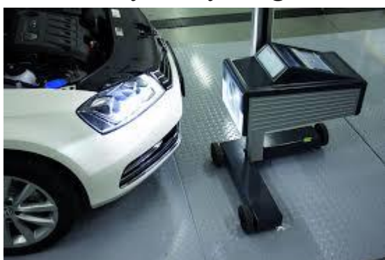
2.43-rasm. Faralarni turli asboblar yordamida sozlash
