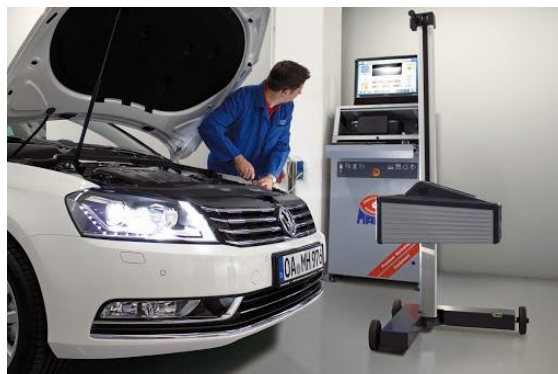
2.43-rasm. Faralarni turli asboblar yordamida sozlash
