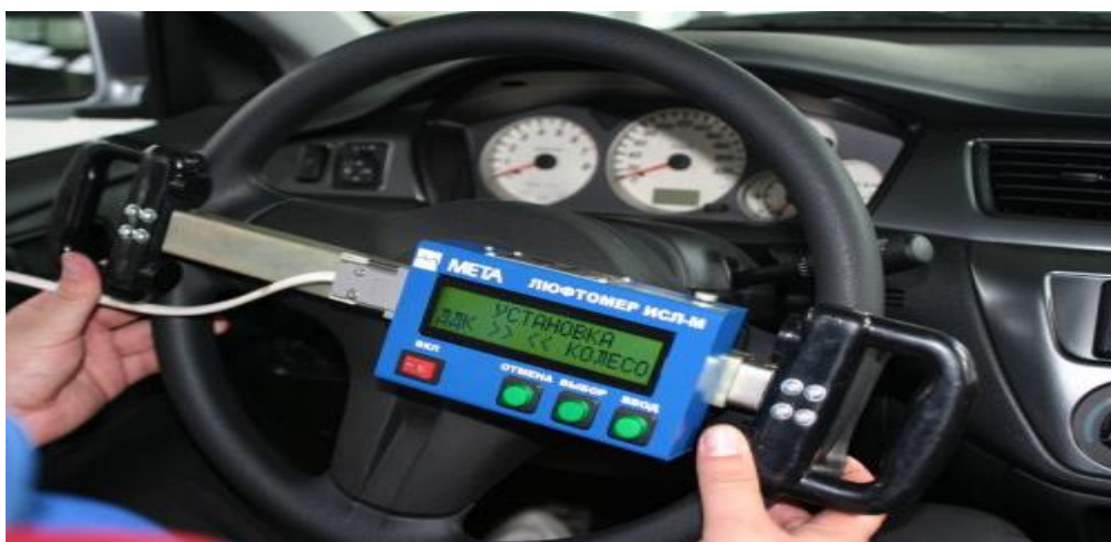
2.55-rasm. Rul chambaragi lyuftomer yordamida aniqlash
