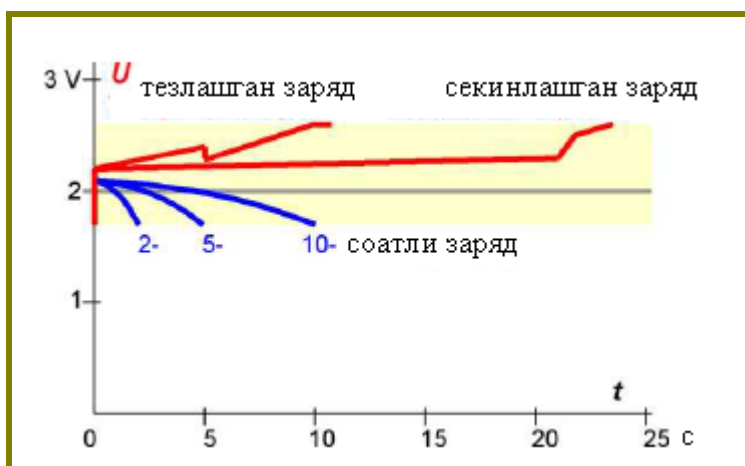
4.14- rasm. Qo'rg'oshinli akkumulyatorni kuchlanishini turli zaryad va razryadda o'lchash.
