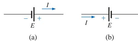
FIG. 4.13 Battery power: (a) supplied; (b) absorbed.
