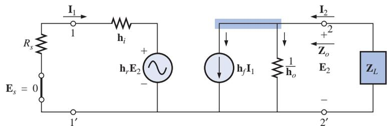
FIG. 26.52 Determining  $\mathbf{Z}_o$  for the hybrid equivalent network.
