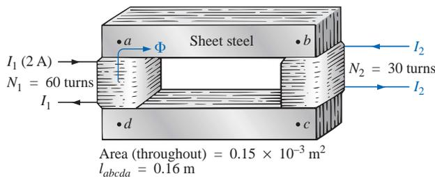
FIG. 11.33 Transformer for Example 11.5.
