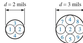
$$A = (2 \text{ mils})^2 = 4 \text{ CM} \quad A = (3 \text{ mils})^2 = 9 \text{ CM}$$
