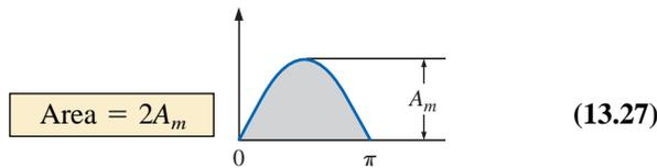
Since we know the area under the positive (or negative) pulse, we can easily determine the average value of the positive (or negative) region of a sine wave pulse by applying Eq. (13.26):
